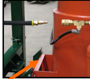
Connect Timer Control Panel Pressure Line to Automatic Purge System
