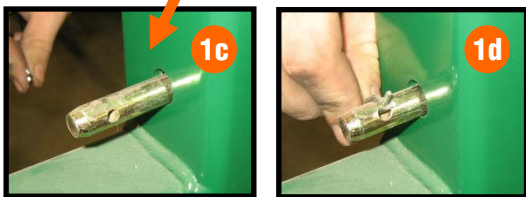
Insert the Frame Locking Pin , secure with clevis pin
