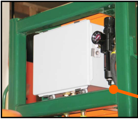
Connect Timer Control Panel Pressure Line to Automatic Purge System
